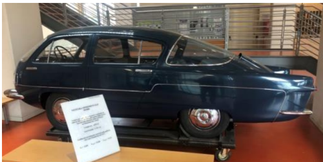
According to the placard, it was designed in 1955 by Alberto Morelli. In 1977 it was placed in the wind tunnel at Pininfarina where it registered a 0.295 Cx.
