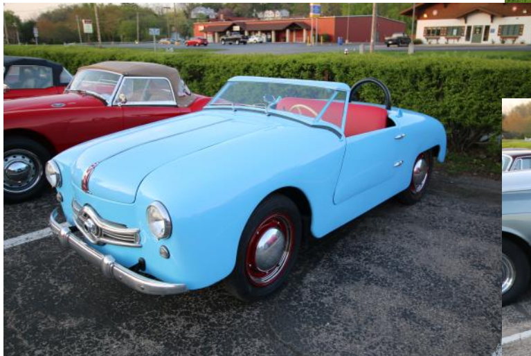
Ted Zamjahn's Panhard Dyna with supercharged flat twin engine.
