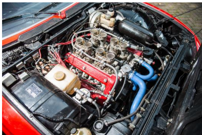
Carb'd Montreal with blue silicon hoses
