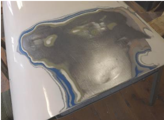
Photo 3. Area sanded and ready for filler
