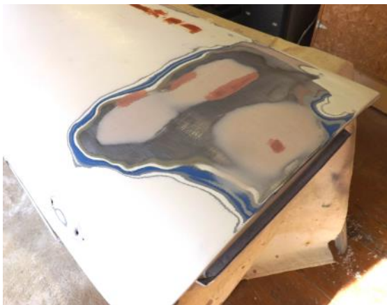
Photo 4. Filled and spot putty applied
