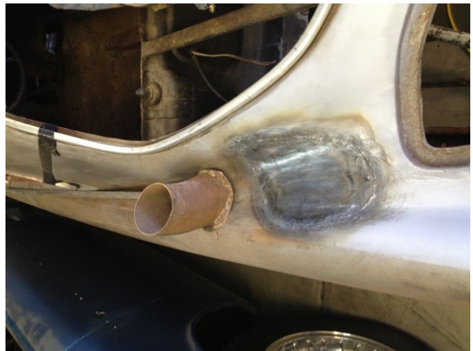
Rear fender hole patch and mystery inlet pipe
