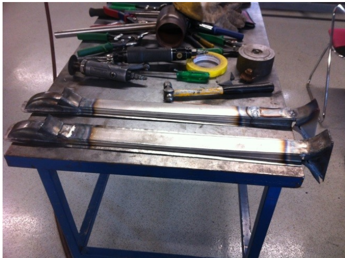
Creative bending, cutting, welding & voila! Gas tank support frames
