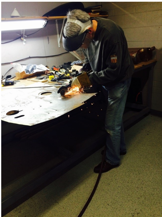
Cutting the slot for the Veloce gas tank breather tube
