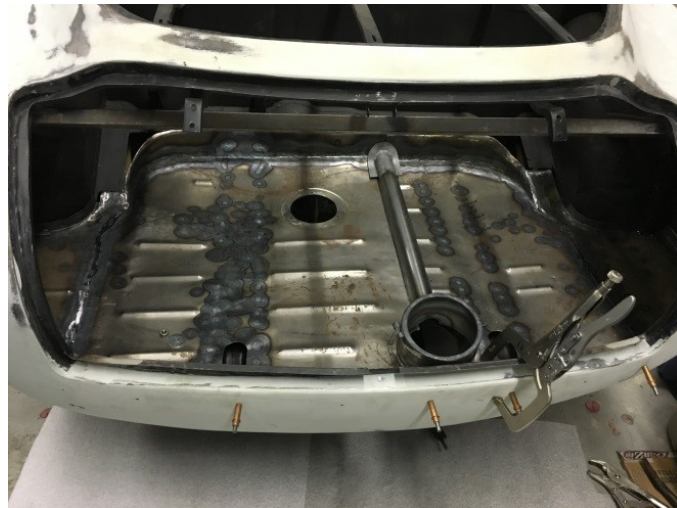
Clecos and clamps soon to be replaced with weld
