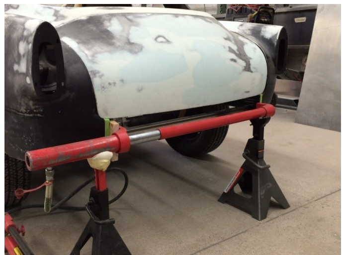
Lower valance was so poorly installed that it pulled the rear sheet metal out of shape so that the trunk lid no longer fit. Valance was cut away, a stretcher used to bring the car back into shape, and then the valance panel re-installed.
